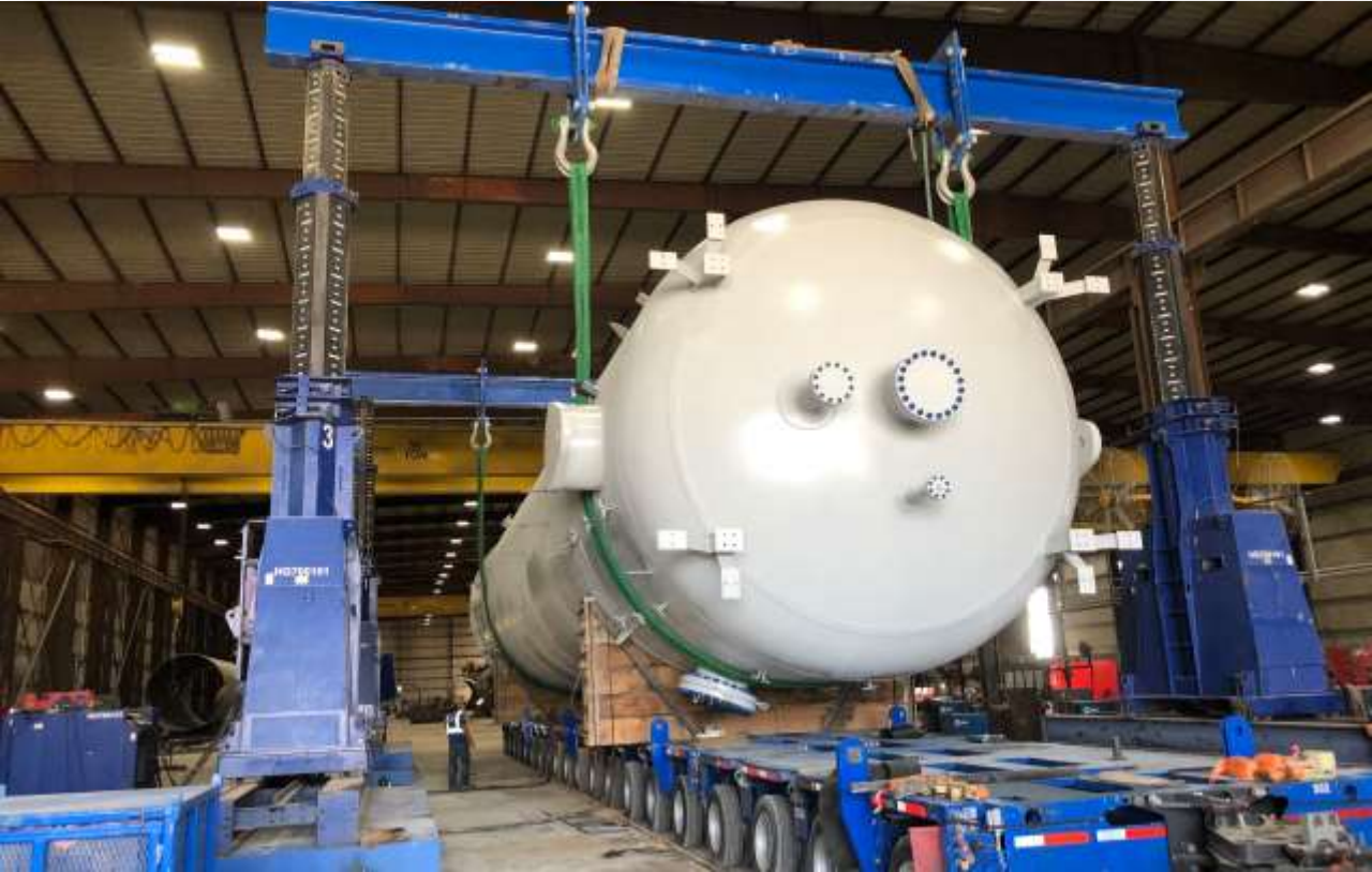
621,240lbs HP Fuel Gas Mixing Drum
